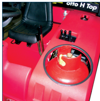
LPG systeem Installation GPL
